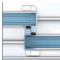
Moving of the leafs using a telescopic system
